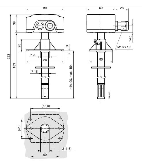
Drilling plan with (without) mounting flange
